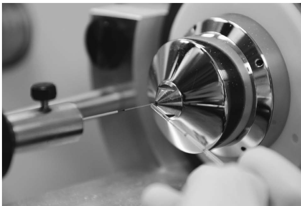
FIGURE 12. Measuring the flow rate through the microcapillary FSC HPLC column using a calibrated glass capillary pipette.
