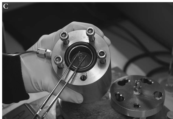
FIGURE 7. (A) Diagram of the pneumatic loading device, “loading bomb,” for packing microcapillary FSC HPLC columns. (B) Actual loading bomb on a stir plate. (C) Using tweezers to insert a glass vial containing the methanol-reverse phase resin slurry for packing the FSC column. The vial contains a microstir bar for keeping the slurry in suspension while the column is packing.
