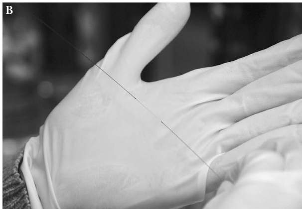
FIGURE 5. (A) Using a methanol-soaked Kimwipe, gently wipe clean the charred black plastic coating from the FSC to expose the quartz glass. (B) Exposed quartz glass of an FSC ready for pulling into micro-capillary HPLC columns using the laser puller.
