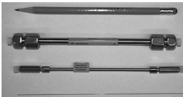
FIGURE 2. Different size RP-HPLC columns used for LC-MS/MS experiments. For RP-HPLC, a 4.6-mm, 1-mm, and 0.1-mm inner diameter column can be used. For high-sensitivity proteomics LC-MS/MS experiments, the 0.1-mm or 100- \mu\text{m} fused silica capillary (FSC) column, shown at the bottom of the figure, is typically used.
