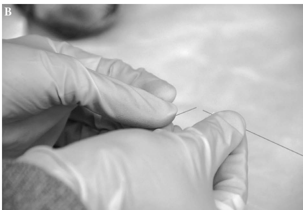
FIGURE 3. Cleaving fused silica capillary (FSC). (A) A silica scribe is used to lightly score the FSC. (B) After the plastic coating and quartz glass are scored with the silica scribe, the FSC will break into two pieces with a light force.
